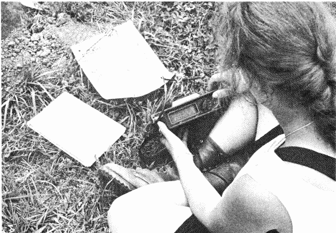
Figure 5. During an archeological survey of the development zone at Russell Cave National Monument, Alabama, a global positioning system was used to determine the exact locations of archeological sites. NPS archeologist Margo Schwadron is shown here recording the digital readout (electronic signals beamed from several satellites) of the coordinates of a Woodland and Archaic period site in the park. (Southeast Archeological Center, NPS)
